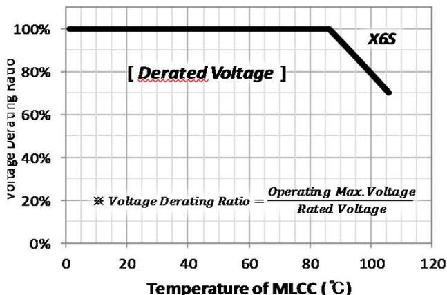
This product, which guarantees High Temperature Reliability Test with 100% of rated voltage at the maximum temperature, is recommended to be used in the circuit with derated voltage compared to the rated voltage of the capacitor for long lifetime.
