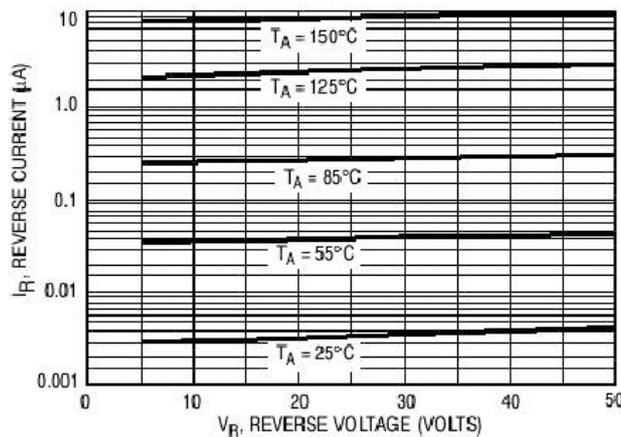
Figure 2. Leakage Current
