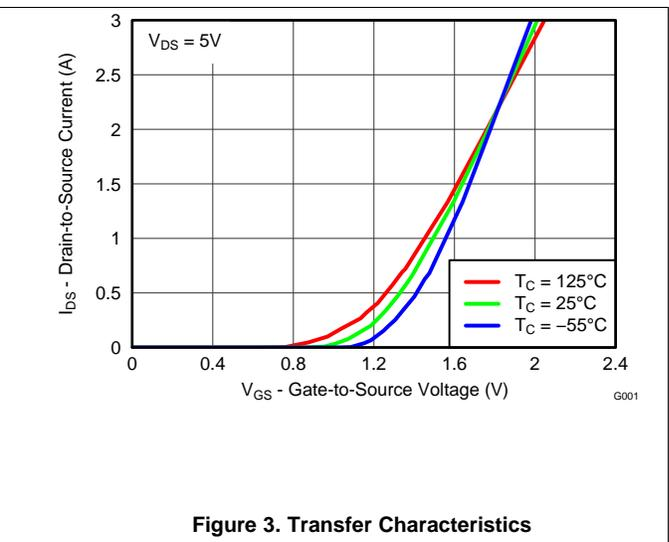
Figure 3. Transfer Characteristics
