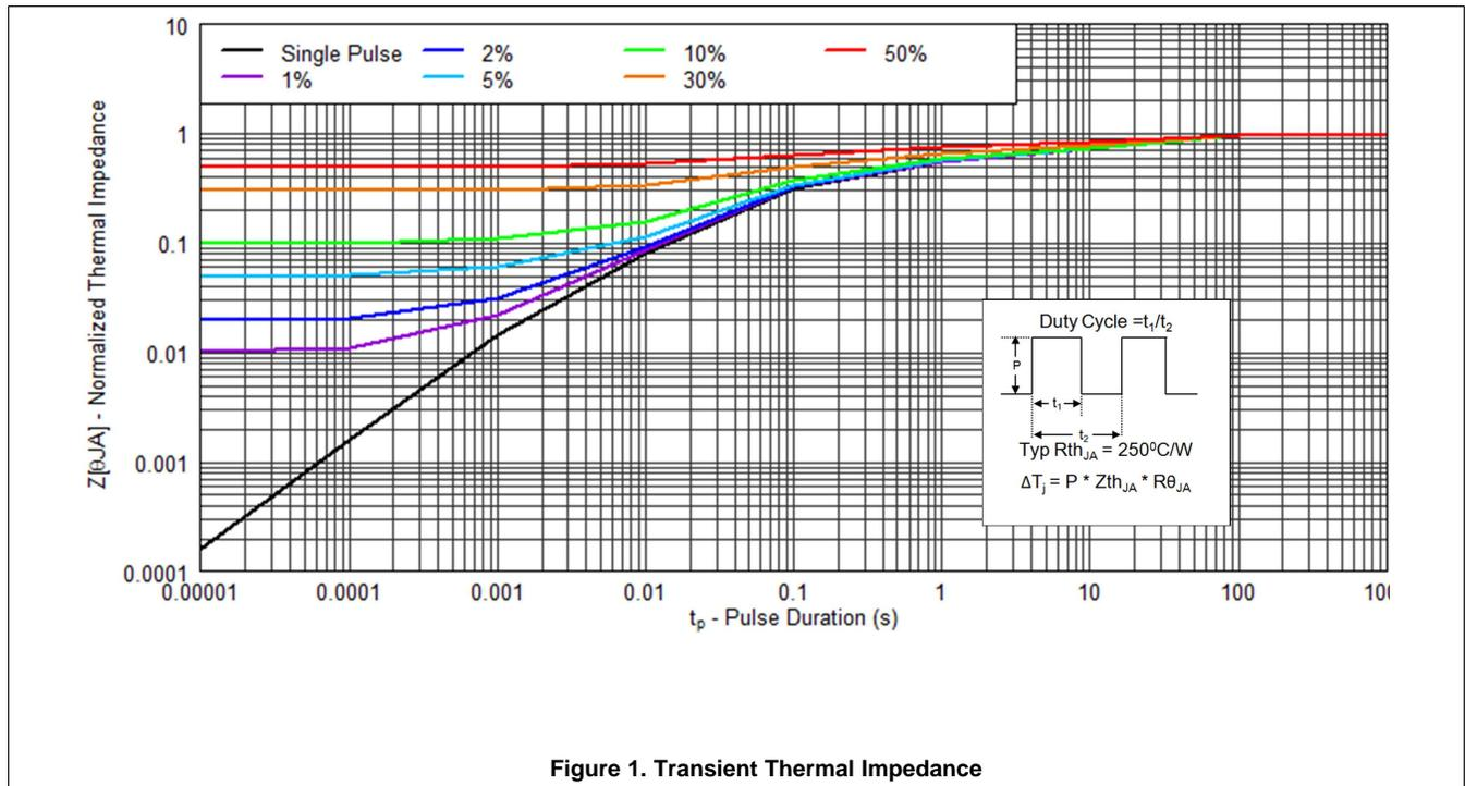
Figure 1. Transient Thermal Impedance
